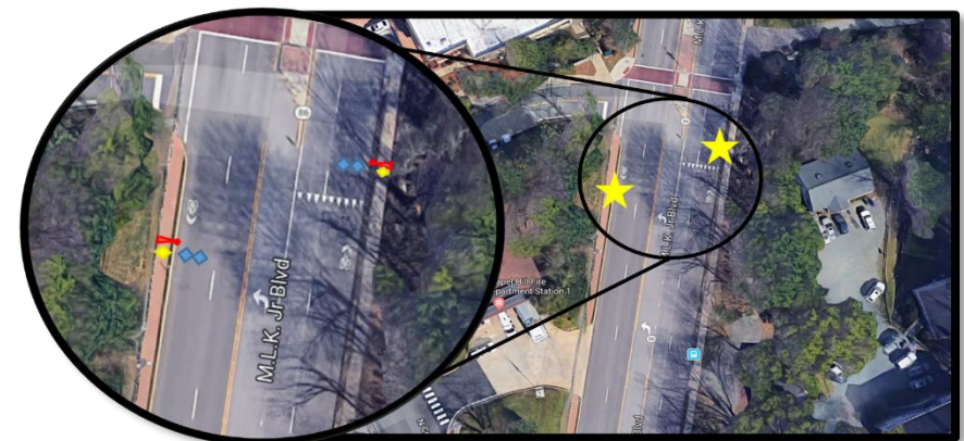
Figure 2. Site diagram showing bicycle and pedestrian count equipment placement
