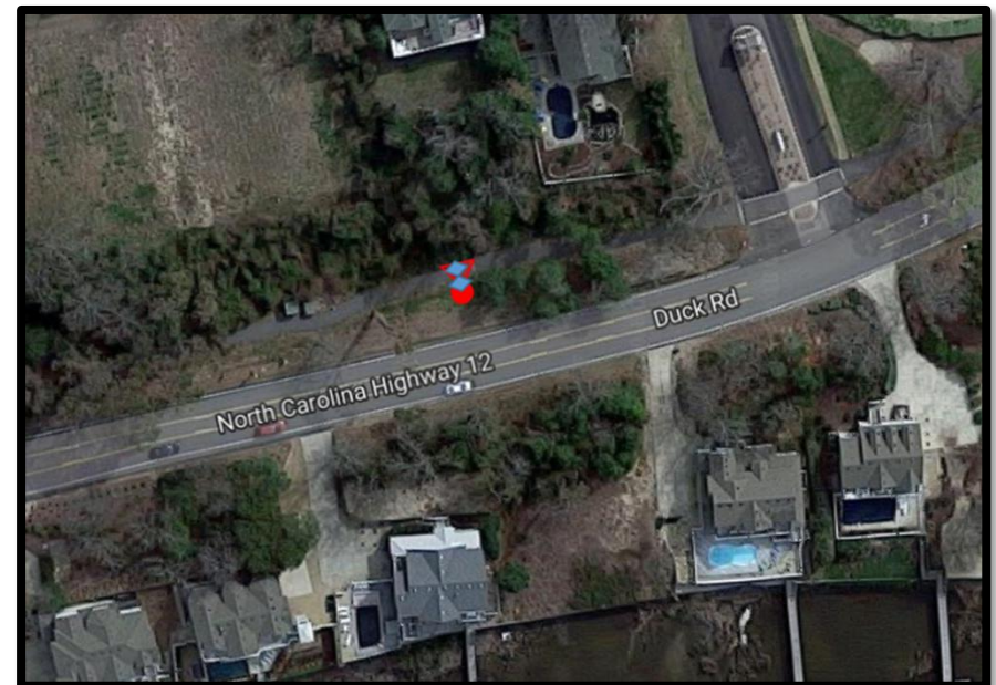
Figure 2. Site diagram showing bicycle and pedestrian count equipment placement (Left is north)
